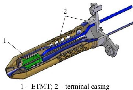
Figure 2. Xenon- fueled ETMT manufactured by SSTL
