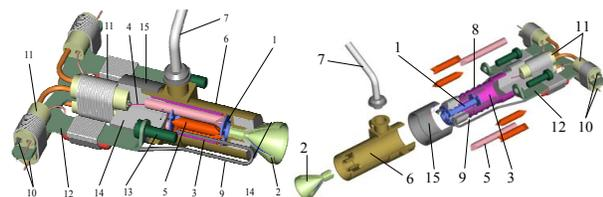
1 – gas duct; 2 – detachable nozzle; 3 – liner; 4 – heating elements; 5, 11 – two-channel ceramic tubes; 6 – chamber; 7 – ammonia feeding line; 8 – spring swirler; 9 – thermocouple; 10 – terminals; 12 – terminal casing; 13 – screws; 14 – sealant; 15 – extension.
