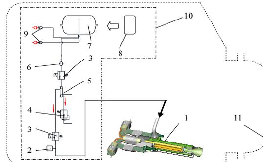
Figure 12. Scheme for testing ammonia-fueled ETMT with THE in a vacuum chamber
