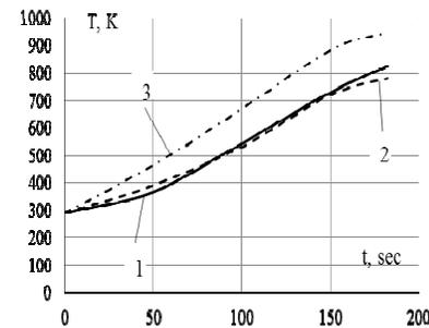
1 – ETMT with cylindrical terminal casings having gas duct length of 29 mm (Figure 12); 2 – ETMT with flat terminal casings having gas duct length of 29 mm (Figure 14); 3 – ETMT with flat terminal casings having gas duct length of 16 mm (Figure 16).
