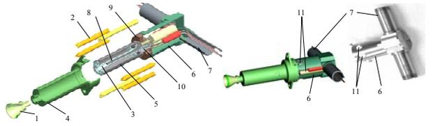
1 – detachable bell nozzle joinable with gas duct; 2 – THE; 3 – gas duct; 4 – outer casing; 5 – inner casing; 6,7 – main and additional terminal casings; 8 – thermocouple; 9 – nut; 10 – ETMT sealing zone; 11 – sealing holes.
