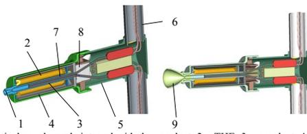
1 – conical nozzle made integral with the gas duct; 2 – THE; 3 – gas duct; 4 – casing (outer and inner); 5 – main terminal casing; 6 – casing for additional terminals; 7 – thermocouple; 8 – ETMT sealing point; 9 – detachable bell nozzle.
