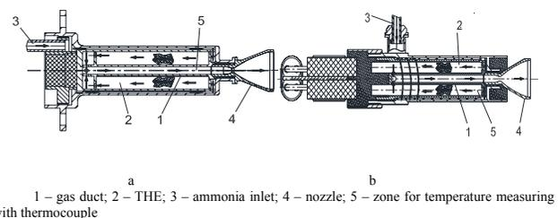
1 – gas duct; 2 – THE; 3 – ammonia inlet; 4 – nozzle; 5 – zone for temperature measuring with thermocouple
