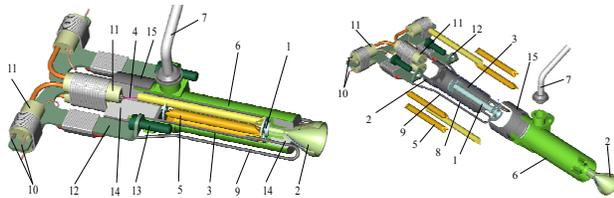
1 – gas duct; 2 – detachable nozzle; 3 – liner; 4 – heating elements; 5, 11 – two-channel ceramic tubes; 6 – chamber; 7 – ammonia feeding line; 8 – spring swirler; 9 – thermocouple; 10 – terminals; 12 – terminal casing; 13 – screws; 14 – sealant; 15 – extension.
