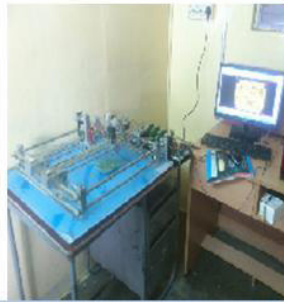
proposed flexible flying board machine connected with the PC
