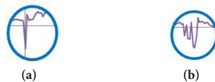
Figure 7. Snippet from response of accelerometer differentiating gradual and high braking intensity, (a) Gradual slope and (b) Steep Slope.
