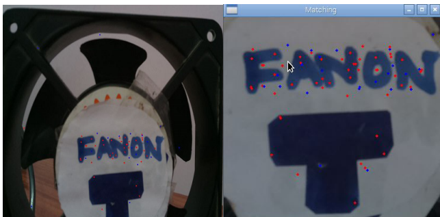
Figure 8. Template matching using SURF.
