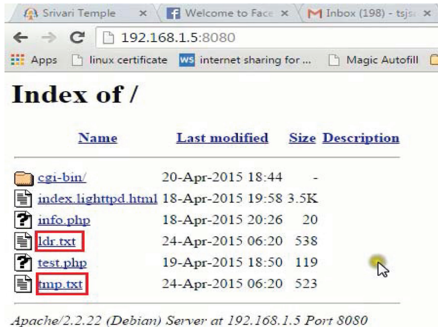
Figure 6. Sensor values stored as log files in web server.
