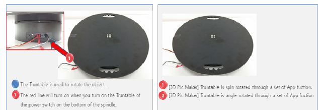
Figure 10. Turntable power on/off function (left), Turntable rotated function (right).
