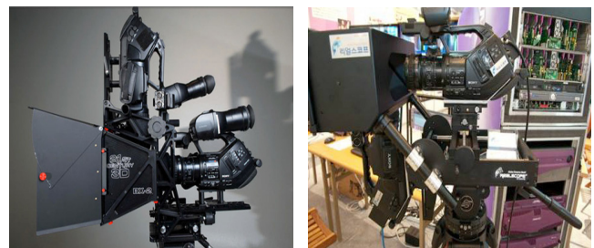
Figure 2. Beam split rig.
