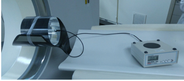
Figure 2. An equipment for measuring CT dose and ionization chamber.
