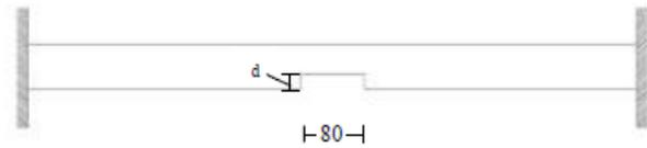
**Figure 1.** Thickness reduction at damage location.
