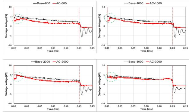
**Figure 3.** Discharge voltage characteristics according to engine speed (rpm).
