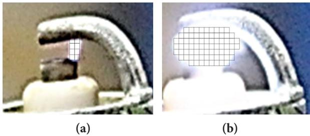
**Figure 4.** Comparison of ignition cross sections at 800rpm (a) Point ignition and (b) AC power ignition.
