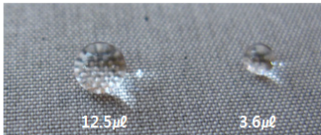
Figure 6. Photograph image of water droplets on a 50D sample treated with Fluoro-C2.
