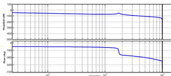
Figure 5. Bode of the discrete system PI controller.
