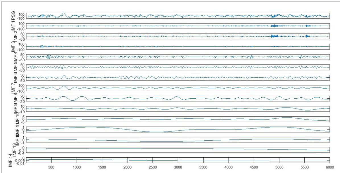
**Figure 2.** IMFs obtained from EEMD process
