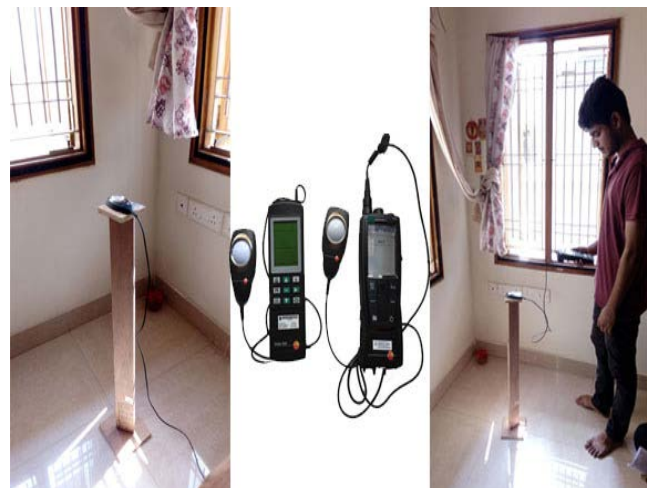
Figure 4. Day lighting measurement.
