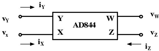
Fig. 5. Proposed current conveyor (AD844) based scheme for the generation of sinusoidal wave form
