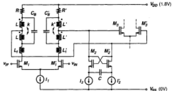
Fig. 9. CMOS implementation of a low-power burst-mode laser driver based on (Eduard *et al.*, 2000).
