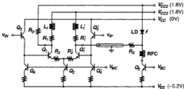
Fig. 6. BJT/HBT implementation of a differential 40 Gb/s EAM-driver output stage with built-in MUX based on (Moller et al., 1998).
