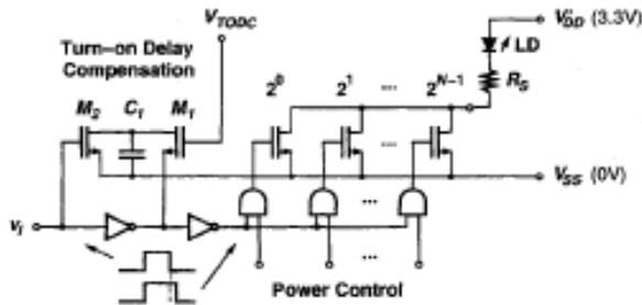
Fig. 10. CMOS implementation of an LED-driver output stage with preemphasis based on (Shieh *et al.*, 2000).
