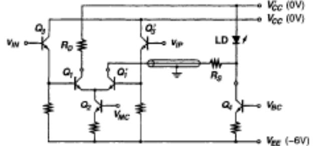
Fig. 5. BJT/HBT implementation of a laser-driver output stage with back termination based on (Runge et al., 1992).
