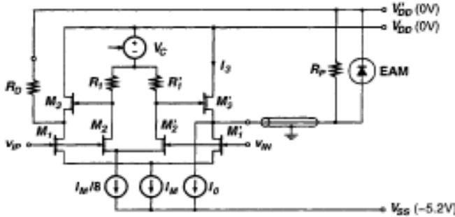
Fig. 4. BJT/HBT implementation of a laser-driver output stage based on (Rein et al., 1988).
