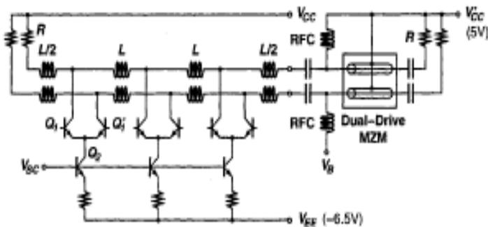
Fig. 8. CMOS implementation of a predriver based on (Galal et al., 2003).
