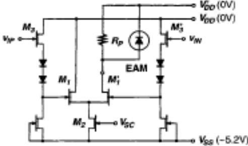
Fig. 2. MESFET/HFET implementation of an EAM-driver output stage with back termination based on (Lao et al., 1998).
