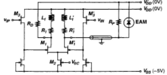
Fig. 3. MESFET/HFET implementation of an EAM-driver output stage with active back termination based on (Ransijn et al., 2001).
