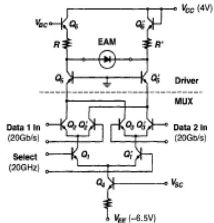
Fig. 7. BJT/HBT Implementation of distributed MZM driver output.
