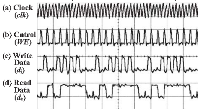
Fig. 6. Measured waveforms at various nodes in 45-nm SRAM with 1K-bit memory cell array incorporating SVL circuit with m of 2 ( f_c=100MHz , V_{dd}=1.8V & V_{ss}=0V ).
