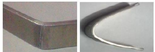
Fig 2. AA2024-AA7075 compressive tested specimens for Taper threaded tool (a) TT1 (b) TT2 and for Straight threaded tool (c) ST1 (d) ST2
