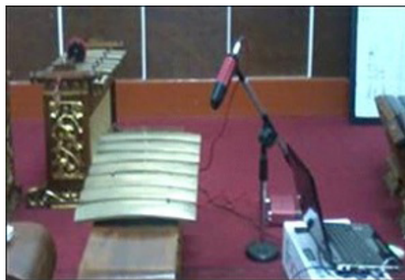
Figure 1. The arrangement of instrument to extract the acoustic data from the OD.
