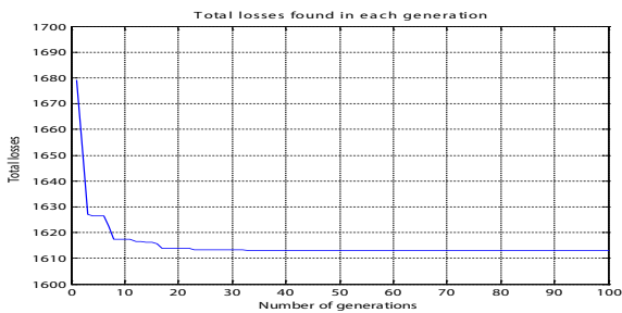
Figure 3. Variation of Total losses (watts) with generations using TS operator.
