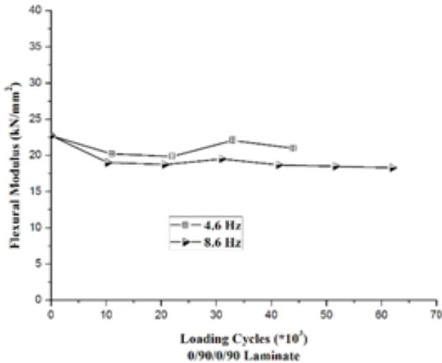
**Figure 11.** Flexural Modulus Variation of 0/90/0/90 laminate.
