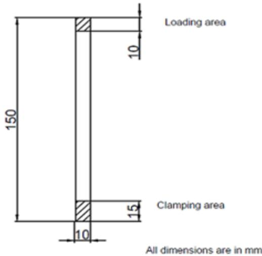
Figure 1. Specimen dimension.
