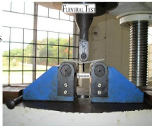
Figure 3. Three point bend test.
