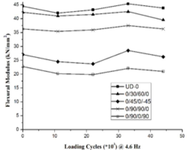
**Figure 12.** Relative Modulus after loading at 4.6 Hz.
