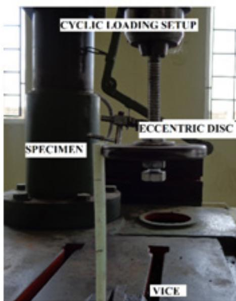
Figure 5. Cyclic loading setup.
