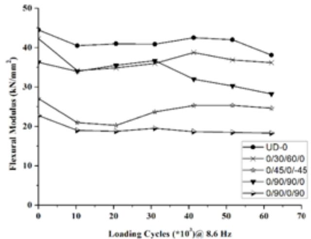
**Figure 13.** Relative Modulus after loading at 8.6 Hz.
