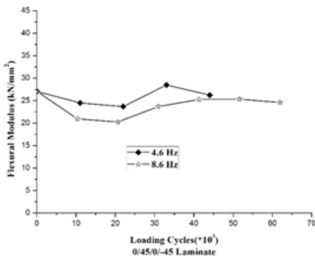
Figure 9. Flexural Modulus Variation of 0/45/0/-45 laminate.
