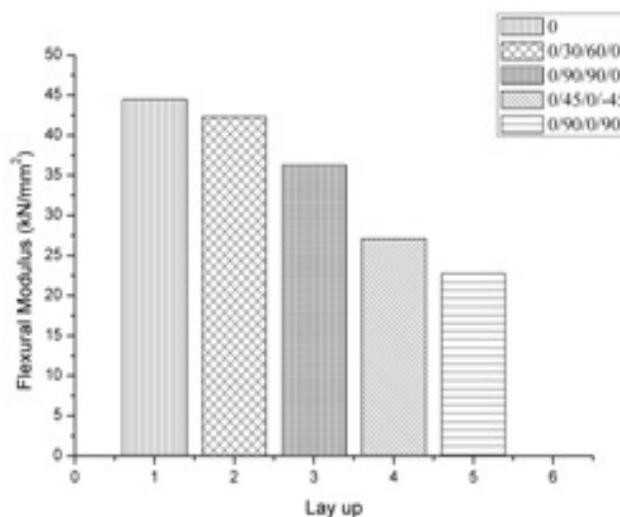
Figure 6. Flexural modulus of virgin specimen.
