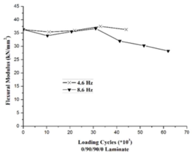
Figure 10. Flexural Modulus Variation of 0/90/90/0 laminate.
