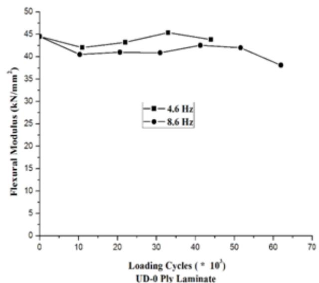
Figure 7. Flexural modulus variations UD-0 ply laminate.
