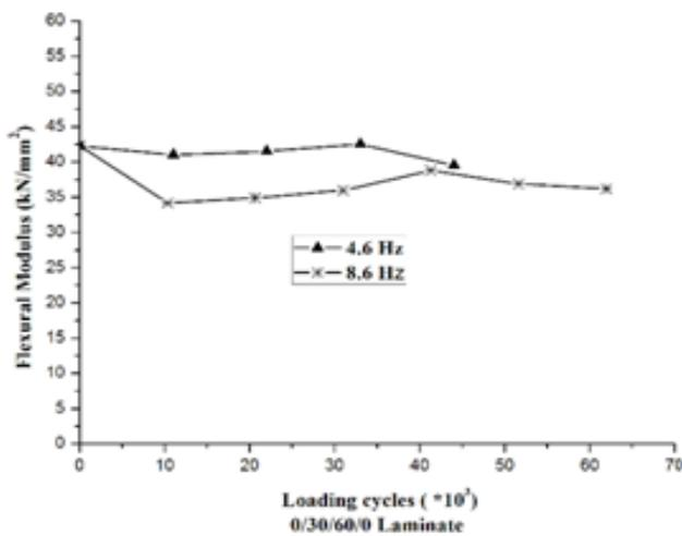
Figure 8. Flexural modulus variation of 0/30/60/0 laminate.
