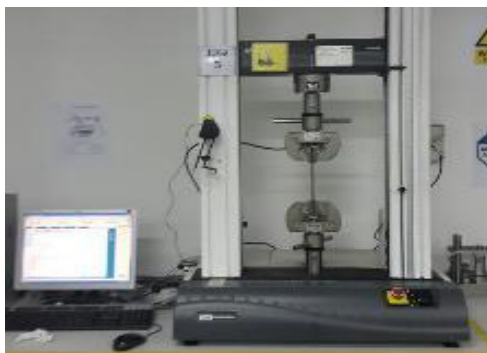
Figure 4. Testing of specimens using UTM.
