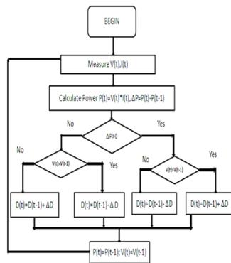
Figure 3. Flowchart of perturb and observe algorithm.
