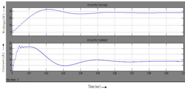
**Figure 5.** Waveforms of PV panel output voltage and current without MPPT.
