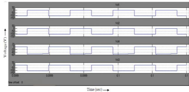
**Figure 8.** Diode voltage stress waveform without MPPT.
