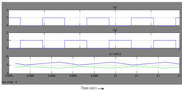
**Figure 6.** Gate pulse of switches and input current of inductor without.
