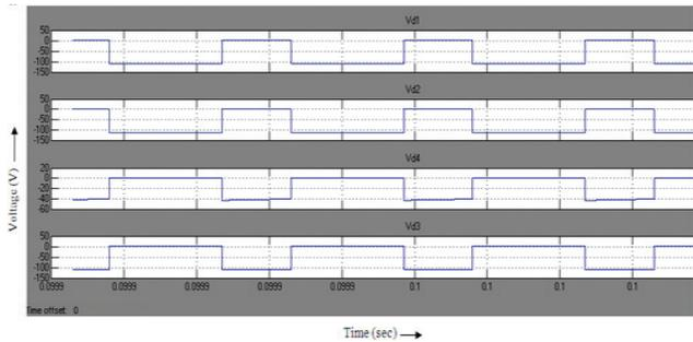
Figure 16. Diode voltage stress waveform with MPPT.
