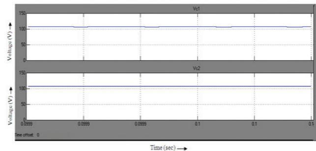
**Figure 10.** Output capacitor voltage stress waveform without MPPT.
