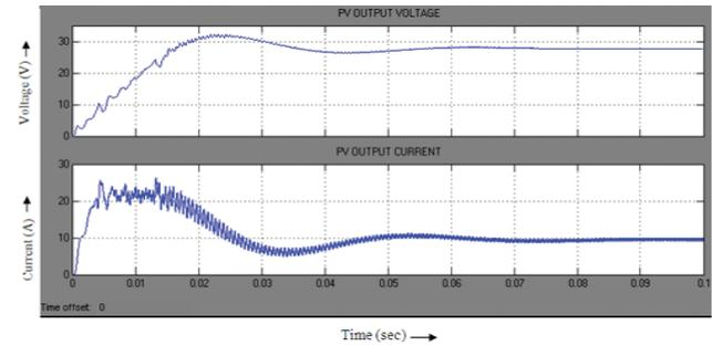
**Figure 13.** Waveforms of PV panel output voltage and current with MPPT.
