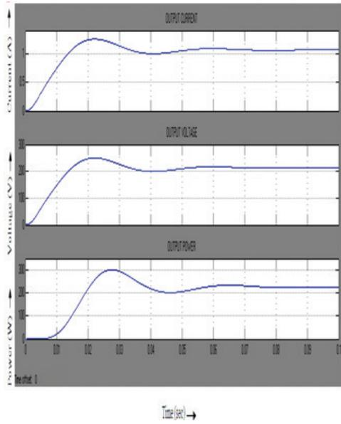
**Figure 11.** Waveform of output current, voltage and power of transformerless interleaved converter without MPPT algorithm.
