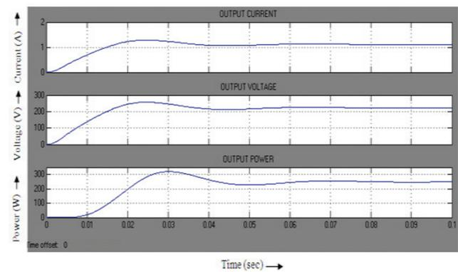
Figure 19. Waveform of output current, voltage and power of transformerless interleaved converter with MPPT.
