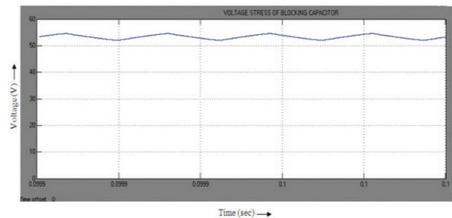
**Figure 9.** Blocking capacitor voltage stress waveform without MPPT.
