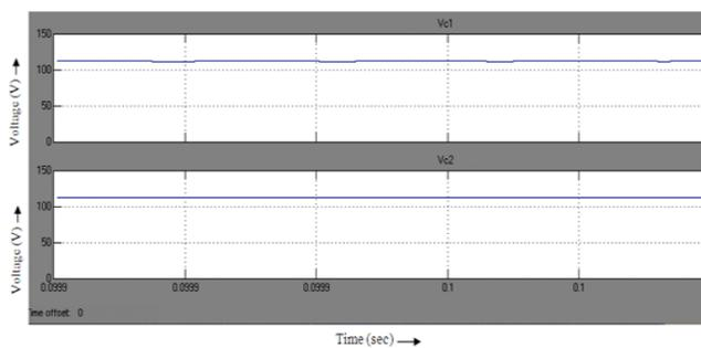
Figure 18. Output capacitor voltage stress waveform with MPPT.
