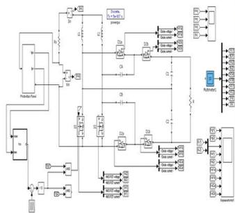
**Figure 12.** Simulation circuit of transformerless interleaved converter with MPPT algorithm.
