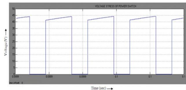
**Figure 15.** Voltage stress waveform of switch with MPPT.
