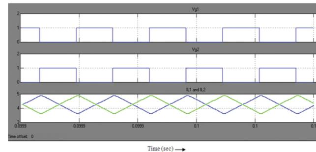
**Figure 14.** Gate pulse to switches and input current of inductor with MPPT.
