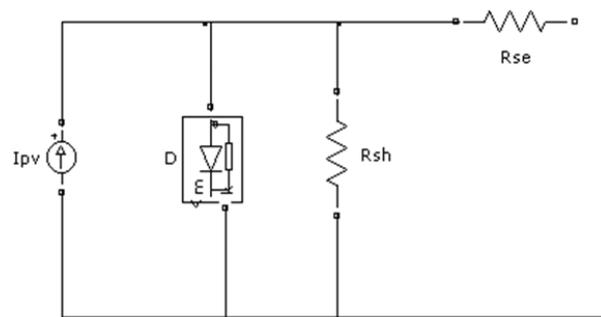
Figure 2. Photovoltaic Model.
