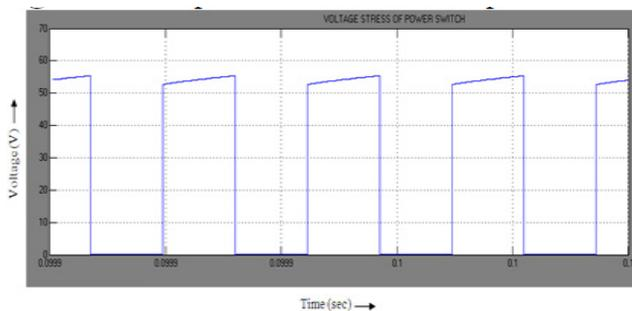
**Figure 7.** Voltage stress waveform of switch without MPPT.
