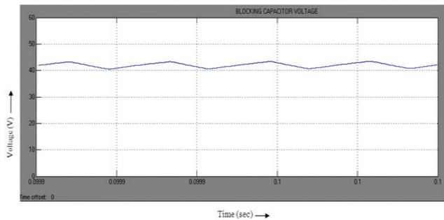
Figure 17. Blocking capacitor voltage stress waveform with MPPT.
