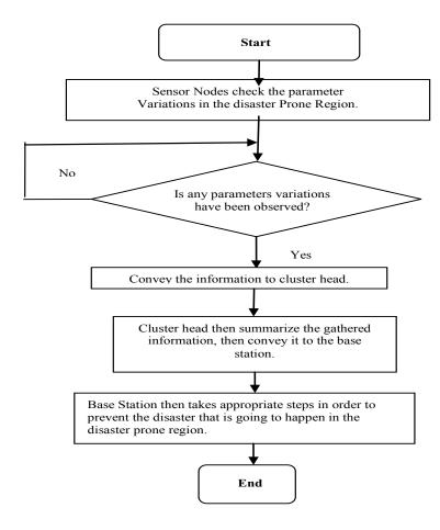
**Figure 1.** Flow chart representing the use of sensor Network in Disaster Prone Region.
