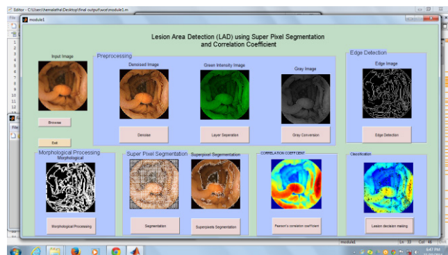
Figure 5. Output showing Lesion Area Detection in intestinal image.
