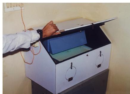
**Fig. 4. *Corcyra* egg sterilization chamber fitted with UV lamp**
