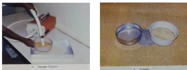
**Fig. 3. *Corcyra* egg cleaning device with vacuum cleaner and sieves**
