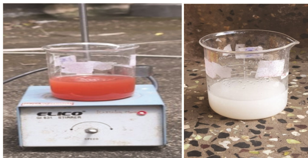
Fig. 8 — Visual observation of before and after degradation of dye
