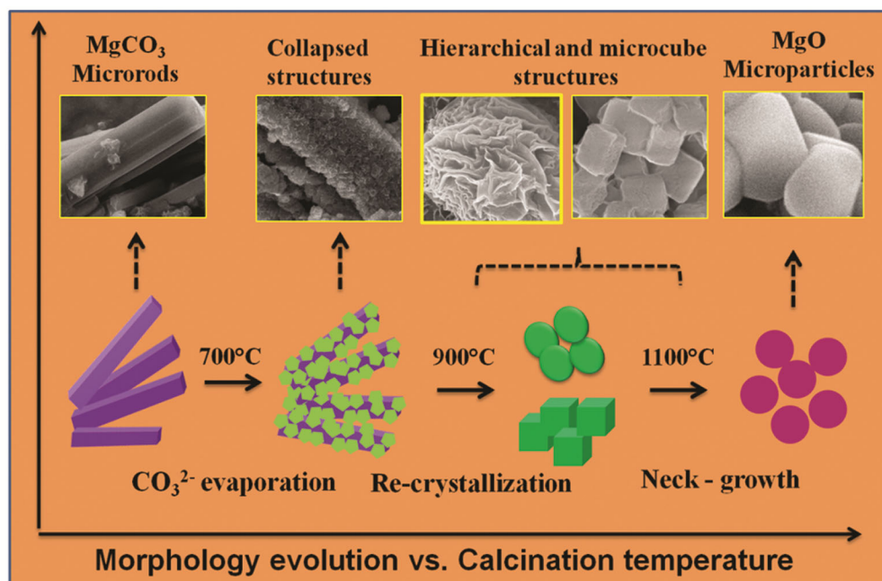
Fig. 6 — Morphology variations as a function of the calcination temperatures
