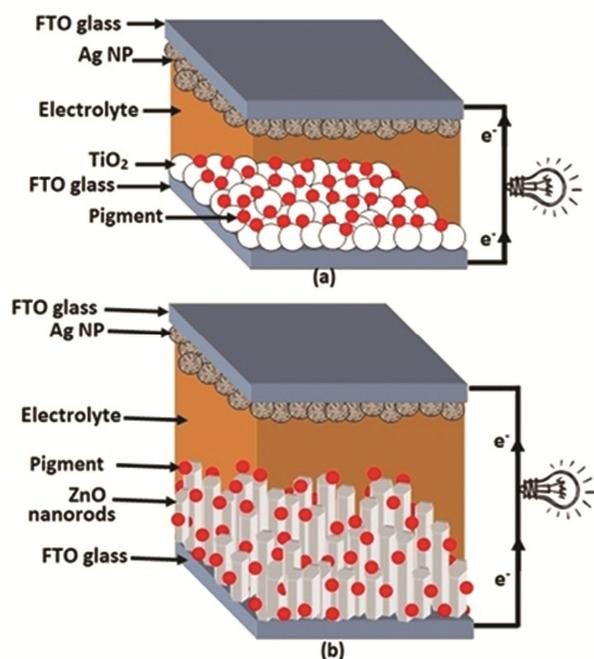
Fig. 1 — BSSC schematic, where photoanode and CE sandwiches a RC. The BSSCs are designed with (a)  $\text{TiO}_2$  based photoanode, where pigments are adsorbed onto  $\text{TiO}_2$  mesoporous film deposited on conducting side of FTO glass (b)  $\text{ZnO}$  based photoanode, where pigments are adsorbed onto  $\text{ZnO}$  nanorod film grown on conducting side of FTO glass
