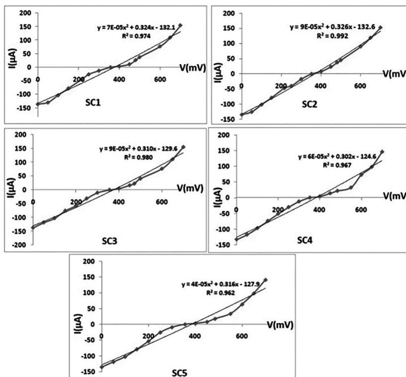
Fig. 4 — I-V characteristics of the DSSCs with ZnO nanorod film
