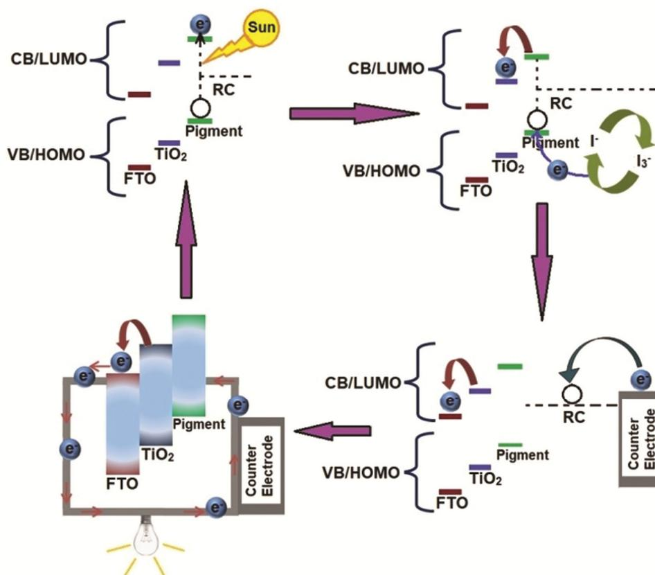
Fig. 9 — Schematic of electron hole pair generation and their transportation through the load using energy band diagram
