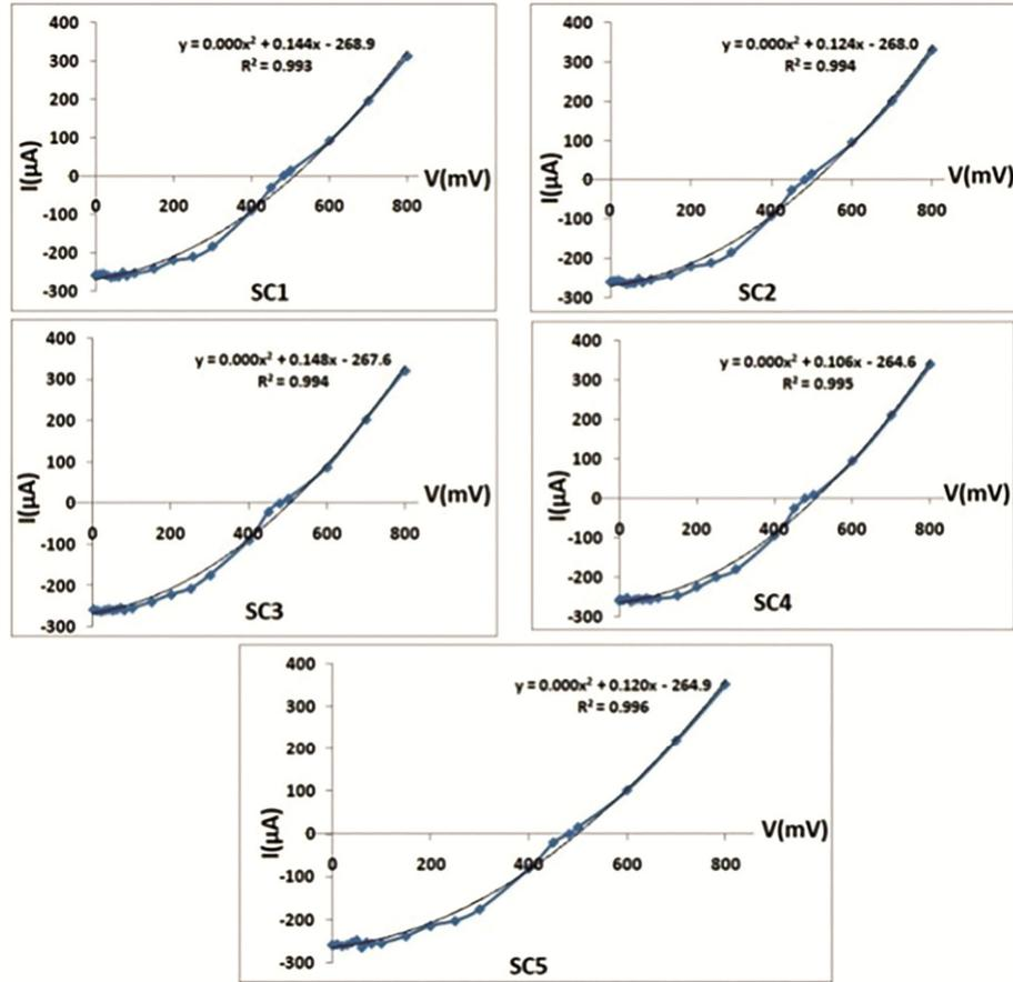
Fig. 5 — I-V characteristics of the DSSCs with TiO<sub>2</sub> mesoporous film
