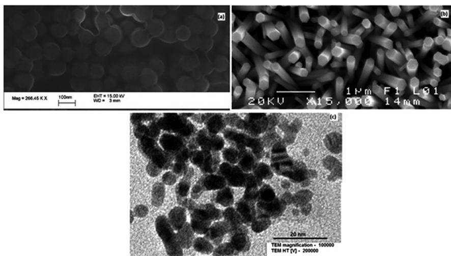
Fig. 3 — Characterization: (a) SEM micrograph of TiO<sub>2</sub> mesoporous film, (b) SEM micrograph of ZnO nanorod film and (c) TEM image of Ag NPs
