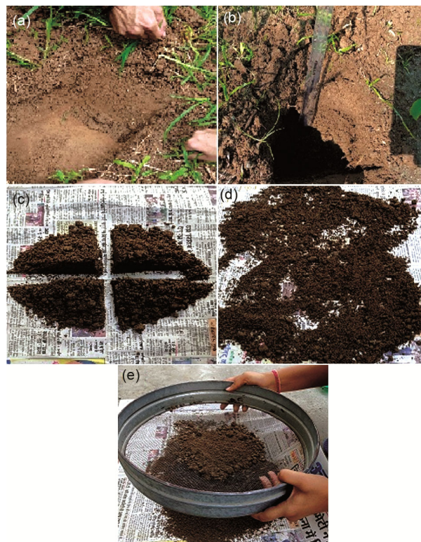
Fig. 2 — (a) Shows V shape hole for sample collection; (b) shows sample collection upto depth 15 cm; (c);(d) shows selection and drying of sample and (e) shows sieving of soil sample.
