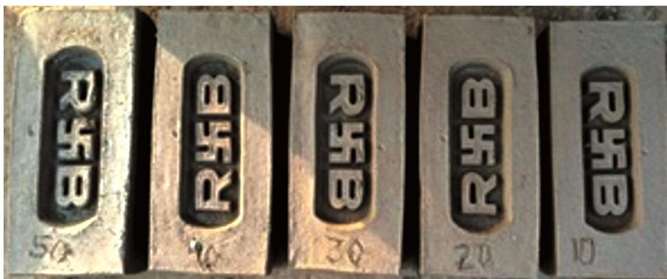
Fig. 1 — Different compositions of clay fly ash bricks.
