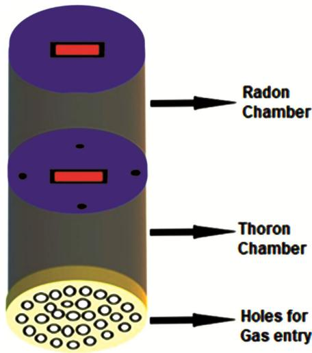
Fig. 2 — Block diagram of pin-hole dosimeter.
