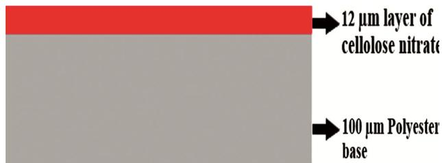
Fig. 1 — Basic schematics of LR-115 SSNTD.
