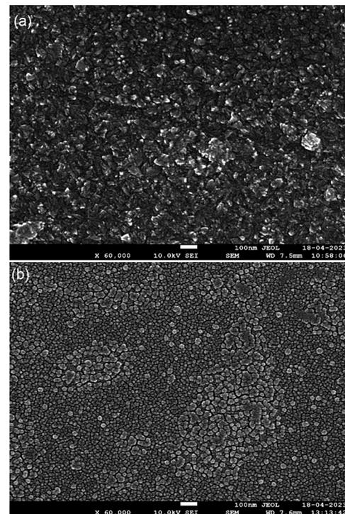
Fig. 2 — FE-SEM images of  $\text{Bi}_2\text{Te}_3$  film deposited onto (a) glass (b) silica substrates.
