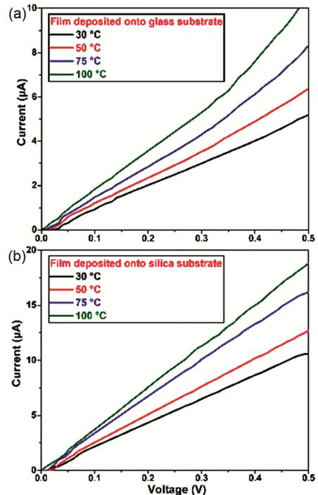
Fig. 4 — Effect of temperature on I-V characteristics of Bi<sub>2</sub>Te<sub>3</sub> film deposited onto (a) glass (b) silica substrates.
