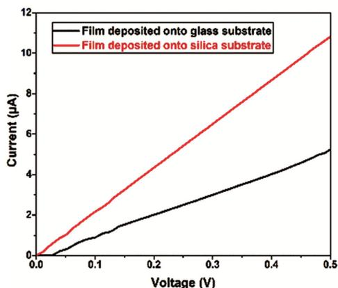
Fig. 5 — Comparison of I-V characteristics of  $\text{Bi}_2\text{Te}_3$  films deposited onto different substrates for temperature  $30\text{ }^\circ\text{C}$ .
