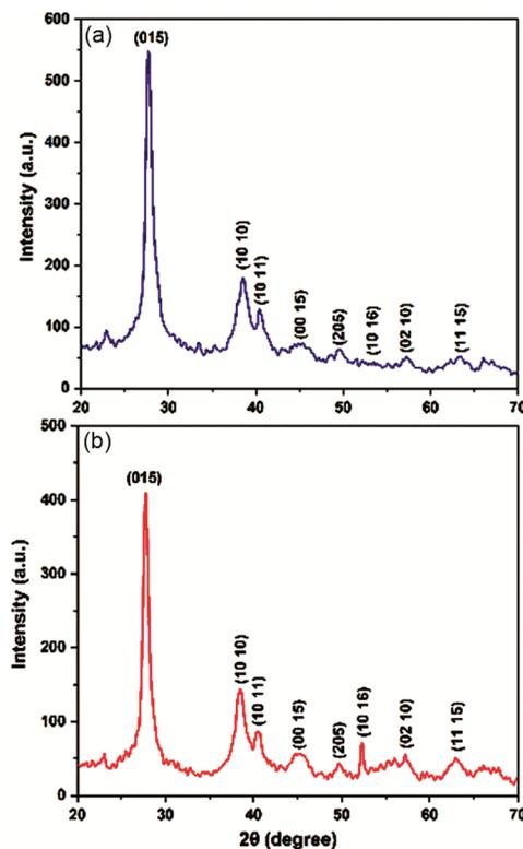
Fig. 1 — XRD spectra of  $\text{Bi}_2\text{Te}_3$  film deposited onto (a) glass (b) silica substrates.
