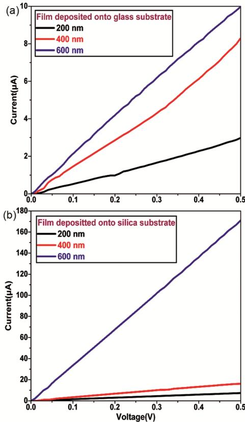
Fig. 3 — Effect of thickness on I-V characteristics of Bi<sub>2</sub>Te<sub>3</sub> film deposited onto (a) glass (b) silica substrates.
