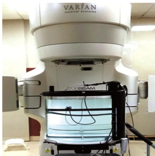
Fig. 2 — Experimental setup used for measurement of unflat (FFF) and flat (FF) photon beams.
