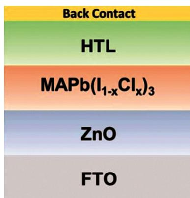
Fig. 1 — Basic device architecture of simulated PSC.
