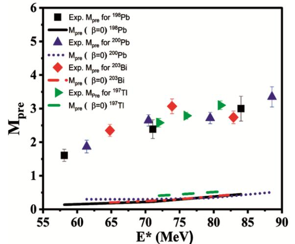
Fig. 7 — Experimental Pre-scission neutron multiplicities ( $M_{\text{pre}}$ ) with statistical model calculations ( $\beta = 0$ ) with inclusion of shell correction in level density and CELD as a function of excitation energy ( $E^*$ ) for  $A \sim 200$ .
