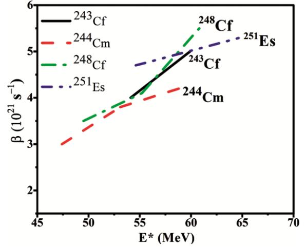
Fig. 10 — Dissipation strength ( $\beta$ ) with inclusion of shell correction in level density and CELD as a function of excitation energy ( $E^*$ ) for mass  $\sim 250$  region.
