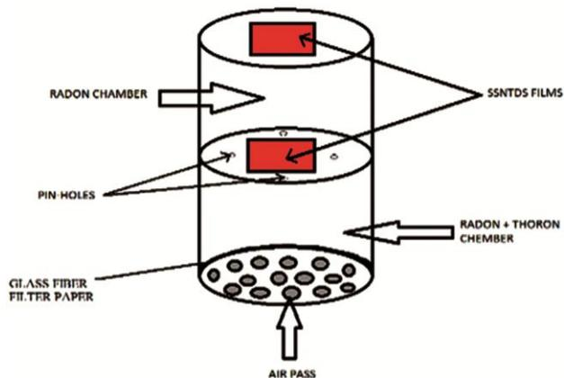
Fig. 2 — Internal schematic diagram of pinhole dosimeter.
