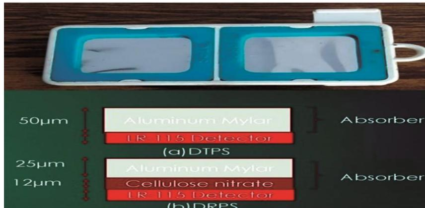
Fig. 3 — Schematic diagram of the DRPS and DTPS.
