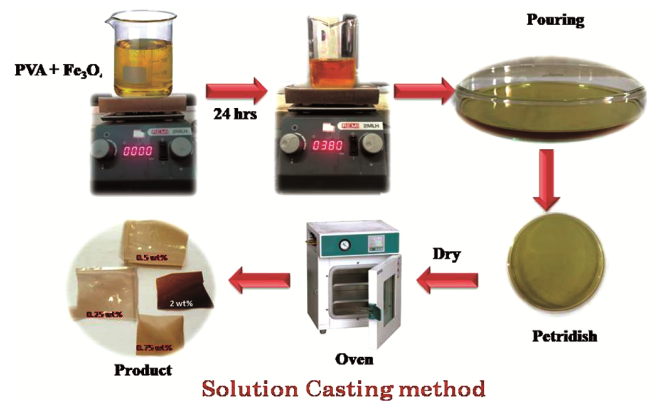
Fig. 3 — Process of solution casting method.
