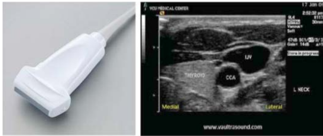
Figure 14. Linear array probe and rectangular display.
