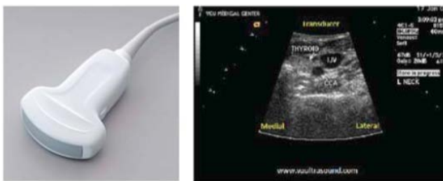
Figure 15. Curved array probe and sector display.
