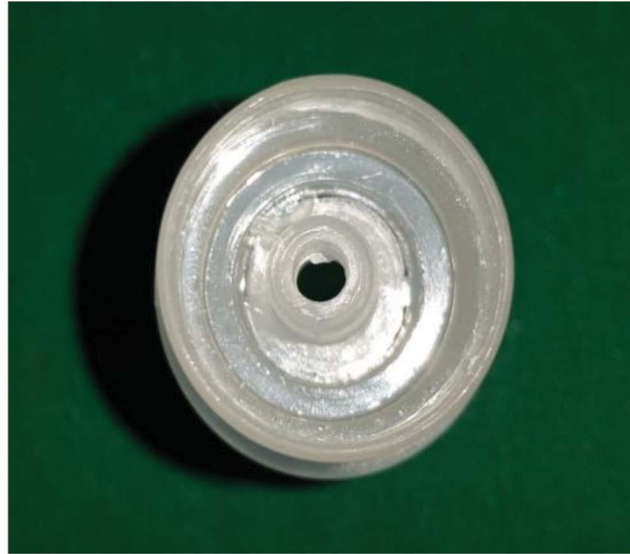
Figure 2. Photograph showing the defective connector with patency for the inner (FGF) and non patency for the outer (corrugated) tubing.
