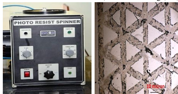
Fig.4 (a) Photoresist unit (b) Micro Pattern just after curing
