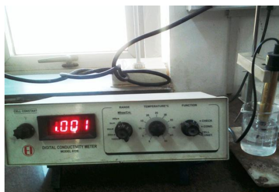
Fig.6 Electrical conductivity of nano/microfluid
