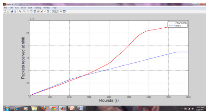
Figure 3. Packets Received at Sink in Base and Proposed Work
