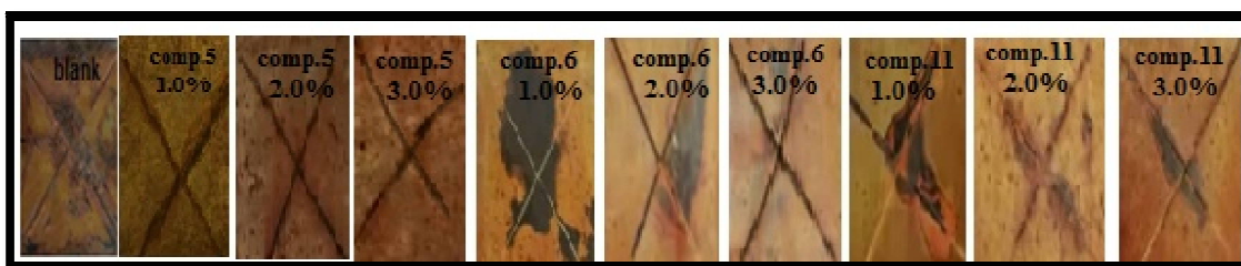
Figure 8: The Photo of the Painted Samples after Exposed to Salt Spray Test (5%NaCl)
