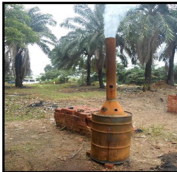
Figure 1: Set Up Drum for Charring of Raw Material
