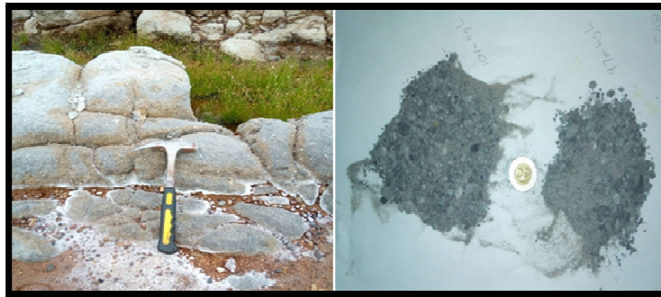
Figure 5: (Left) Outcrop of Keana Formation in Old Awe Town, Note Orthogonal Joint Sets and Efflorescence of Brines Issuing from the Joints (Right) Borehole Sample of Keana Sandstone Collected at about 80m Below Ground Surface
